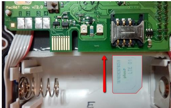
SIM card assembly in MacR6-Z0
